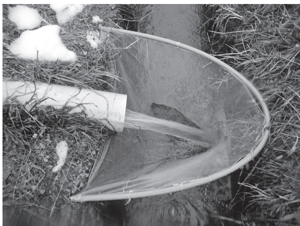
Fig. 3. The fine-meshed, D-shaped net for capturing aquatic animals from the outlet drained.
